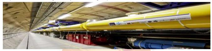
The machine is a superconducting linear accelerator that is housed in a 3.4km-long tunnel complex some 40m beneath Hamburg. It works by accelerating bunches of electrons to almost light-speed, before then throwing them down a slalom course controlled by a system of magnets, known as undulators.
